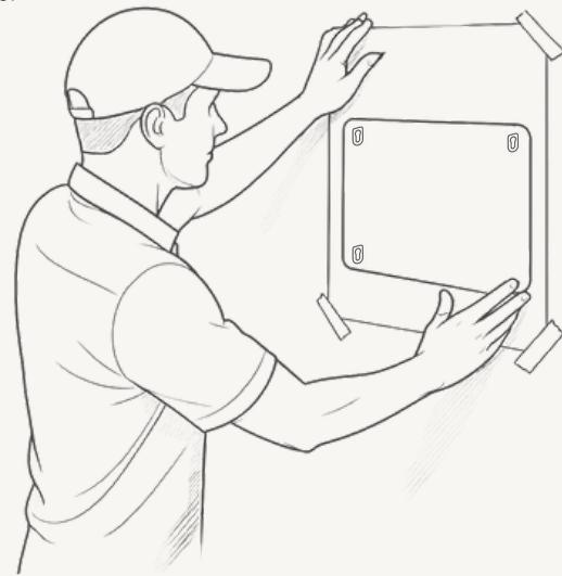
This template ensures accurate positioning and optimal alignment of the kiosk.
